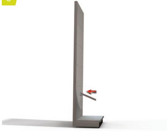
Insert a bracket into the upright "H" slot at an angle as shown above.
